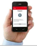
If the identifiers login matches the stored data, the RFID opening medium can be released for opening by touching the medium on the smartphone.
