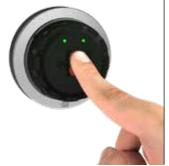
4 Place the RFID opening medium close to the reader area of the lock system and the lock system will open after a valid authorisation.
